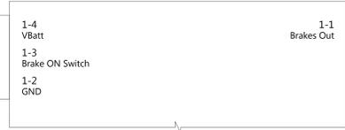
Add mating pigtail - supplied to customer when towing package is selected
