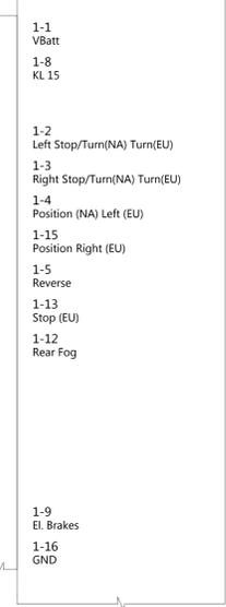
Ground returns from trailer functions are direct to chassis
